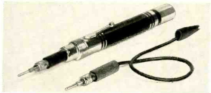
A simple continuity checker of the type shown in Fig. 1. Lamp is in end of probe.
