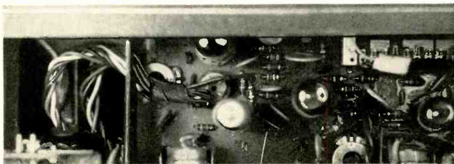
Fig. 3—Part of printed-circuit amplifier used in typical modern tape recorder. All parts are visible, and test points can be reached with long, thin test probe or extension.
